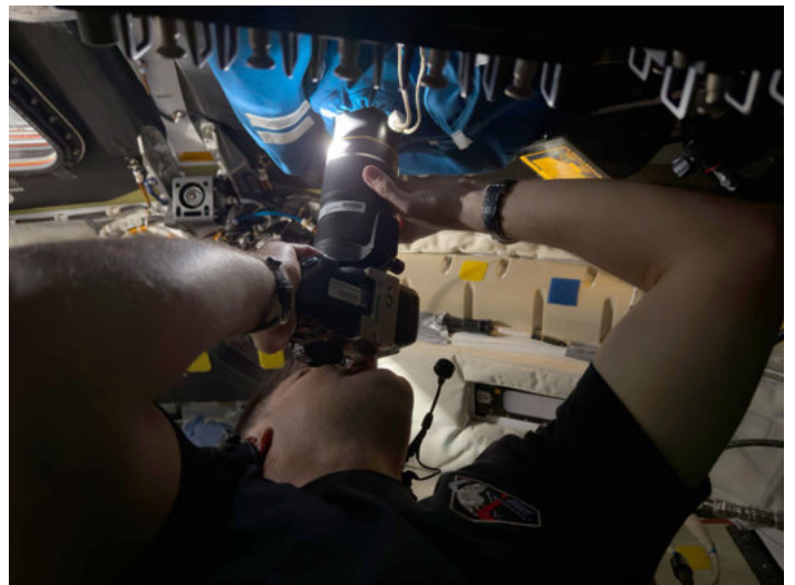
Jeremy Hansen captures an image through the camera shroud covering window 2 of the Orion spacecraft. The camera shroud, essentially a curtain with a hole for the lens to pass through, is used to prevent light from the cabin from reflecting on the window-panes.
