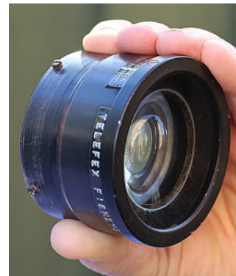
The revised fisheye attachment with better lenses, in a custom engineered aluminium bayonet mount.
