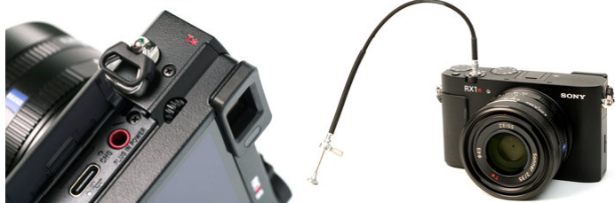
The RX1R MkIII adds a build-in EVF which is much like the A6000 series or the A7Cs. In the head on view you can see how the large eyecup overlaps the rear screen. Top view, with the eyecup removed. Below, size comparison with A6300 and 16-50mm zoom. Above left, USB-C with charging, and mic socket labelled 'Plug In Power' which might confused – means it powers the mic! Above right, the unusual provision for mechanical cable release.
