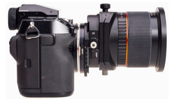
The GF system with its 25mm register and wide throat accepts adaptors for many SLR/DSLR/MF lenses, some with AF. Here a Samyang T/S lens in Canon EF mount is used on a K&F manual adaptor. Below, pixel shift artefacts on a moving detail.
