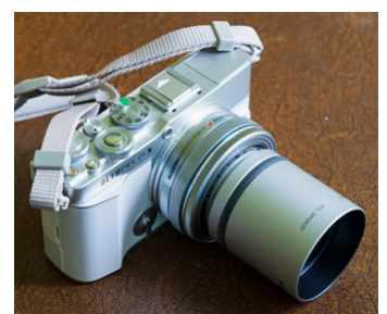
Above, the rear screen articulation – it's good for 'waist-level' or over head viewing of horizontal compositions, or slight angles. But it's almost useless for self-filming as it hangs down behind any tripod mounting! Below, a used 2.5X camcorder tele converter fitted the 37mm thread.
