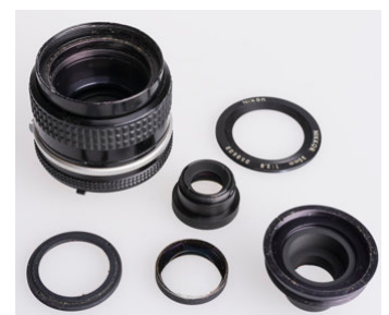
Above right, the Neewer tool's pointed prongs used to unscrew the front element retaining ring. The rear group unscrewed with initial help from the flat blade prongs, then one of the set of rubber cones. These also came in useful hold the optical assemblies (bottom left) as the shape of optical units tend to be either a cylinder or a stepped series of cylinders. The components of the lens during cleaning are laid out below right.
