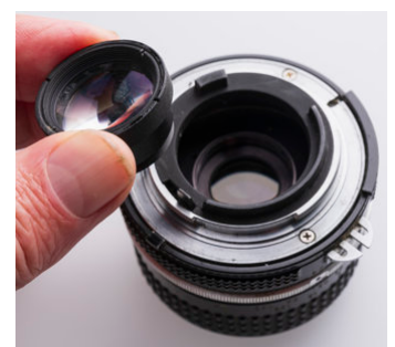
Above right, the Neewer tool's pointed prongs used to unscrew the front element retaining ring. The rear group unscrewed with initial help from the flat blade prongs, then one of the set of rubber cones. These also came in useful hold the optical assemblies (bottom left) as the shape of optical units tend to be either a cylinder or a stepped series of cylinders. The components of the lens during cleaning are laid out below right.
