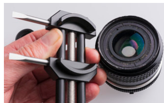
Top, the lens after removing its front bezel, the name and serial number plate which screw into the filter thread until firmly seated. The Neewer Lens Vise tool above is clamped inside the damaged thread by outward pressure and rotated to make it circular again. The rubber cone can then unscrew the bezel.
