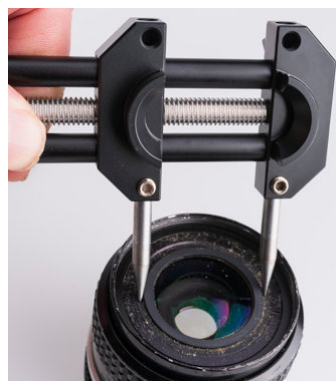
Above right, the Neewer tool's pointed prongs used to unscrew the front element retaining ring. The rear group unscrewed with initial help from the flat blade prongs, then one of the set of rubber cones. These also came in useful hold the optical assemblies (bottom left) as the shape of optical units tend to be either a cylinder or a stepped series of cylinders. The components of the lens during cleaning are laid out below right.
