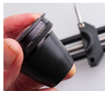
Above right, the Neewer tool's pointed prongs used to unscrew the front element retaining ring. The rear group unscrewed with initial help from the flat blade prongs, then one of the set of rubber cones. These also came in useful hold the optical assemblies (bottom left) as the shape of optical units tend to be either a cylinder or a stepped series of cylinders. The components of the lens during cleaning are laid out below right.
