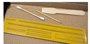
Cleaning out old foam with a small screwdriver and cotton bud with isopropyl alcohol. The re-foam kit is shown below.
