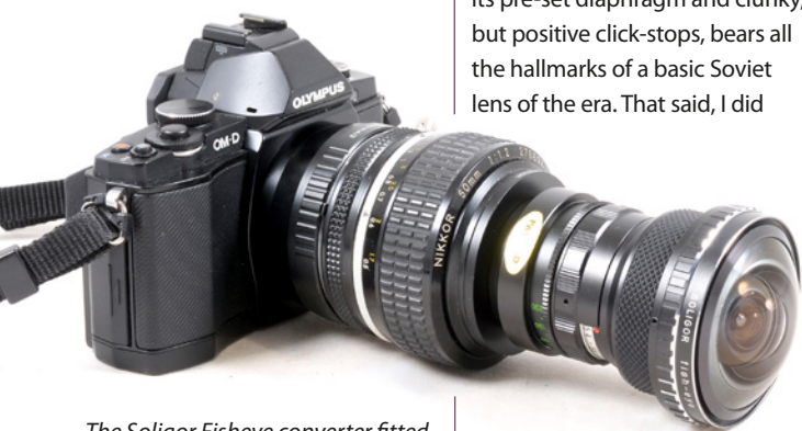
The Soligor Fisheye converter fitted to a 50mm f1.2 Nikkor on Olympus, above; the Peleng 8mm, right.
