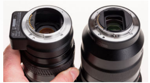
With the E-mount flange in the same position, note how far from the sensor the old DSLR 24-105mm rear element is placed, and how close the rear glass of the FE design can be with the 18mm register. It's this freedom to rethink optical design which has enabled a 24-105mm with near-prime performance (at a price).
