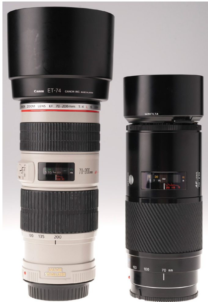
The Canon 70-200mm f 4 IS USM compared in size to the 1985 Minolta 70-210mm f 4 AF. Both are internal zooming, front group focusing designs which do not extend, though the Minolta has a rotating front rim. The Canon focuses down to 1.2m, as does its non-stabilised version, with 0.21X subject scale. The vintage Minolta focuses to 1.1m with 0.25X scale. The Canon weighs 760g (705g for the non-IS version) and is 76 x 172mm in size.
