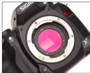
All the Foveon sensor DSLRs from Sigma share the removable IR cut filter mounted behind the lens. This design keeps the sensor itself free from a thick 'filter pack' and has other benefits – see below.
