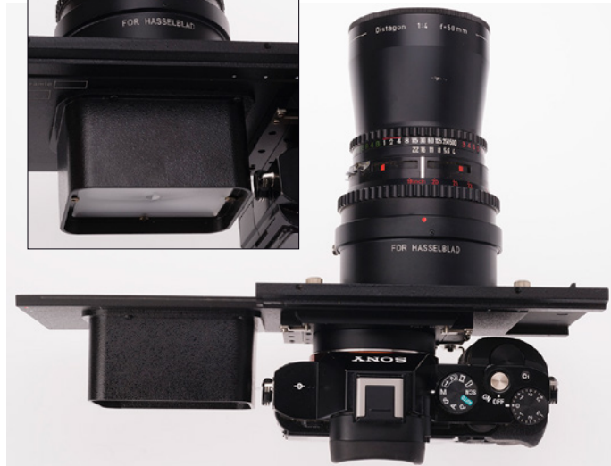
Above: Rhinocam from above showing the A7R body slid to the left.
