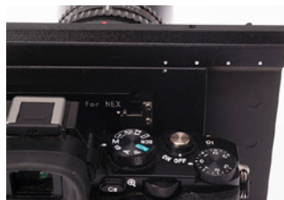
Above: the body dropped to the lowest position. Below left, four marks for sliding APS-C vertical frames; right, the catch for sliding up/down.
