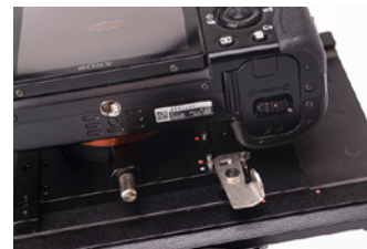
Above: the body dropped to the lowest position. Below left, four marks for sliding APS-C vertical frames; right, the catch for sliding up/down.
