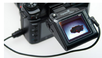
The Seculine ZigView R detects movement on its viewfinder video camera and fires the camera via a dedicated remote cable.
