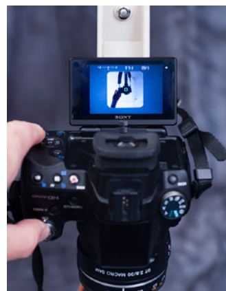
Using the digital centre marking of a live view screen for copy stand alignment with a mirror tile. This also works with EVFs.
