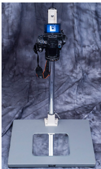
Using the digital centre marking of a live view screen for copy stand alignment with a mirror tile. This also works with EVFs.
